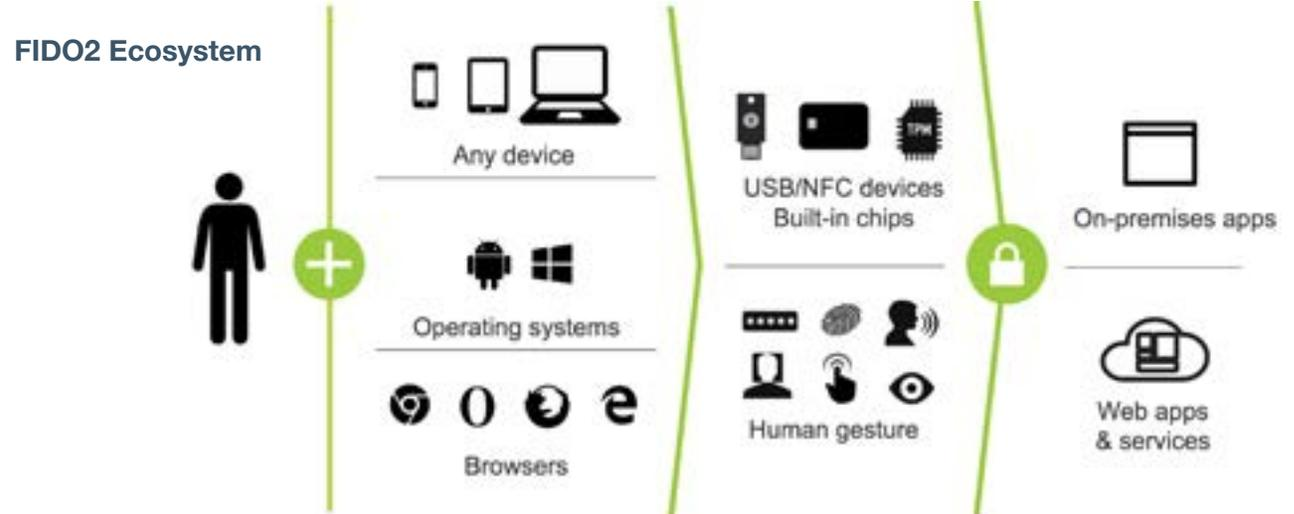
FIDO2 relies on an asymmetric (public/private) pair of cryptographic keys to authenticate users. The public key is stored on any service or computing device supporting FIDO2 authentication, while the private key is kept by the user and is protected on a physical security key, such as the YubiKey 5 Series and Security Key by Yubico. Authentication itself is fast and easy: by simply inserting or tapping the security key the authentication challenge is completed, and login is immediate.
